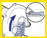
1. Insert tag strip with pins and tag ridge covered by feed horn.
